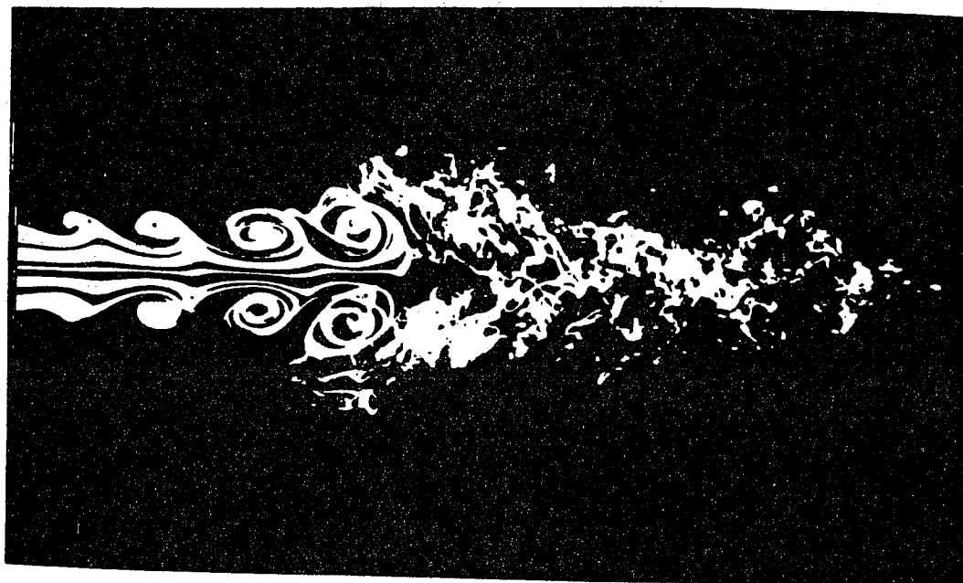
Figure 4-1. Typical jet mean flow profile (a), and evolution of jet turbulence at high Reynolds numbers (b).
