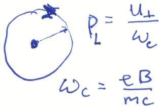
gyration for positive charge particle, as  $\vec{B}$ -field clockwise
