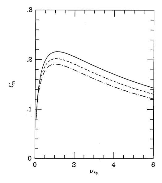
FIG. 1. Plot of the density coupling coefficient to the neoclassical resistivity  $(C_n = -\partial \ln \eta_{\rm nc}/\partial \ln n_e)$ , in terms of  $\nu_{*e}$  for (i)  $\epsilon = 1/4$  (solid line), (ii)  $\epsilon = 1/5$  (dashed line), and (iii)  $\epsilon = 1/6$  (dash-dotted line).
