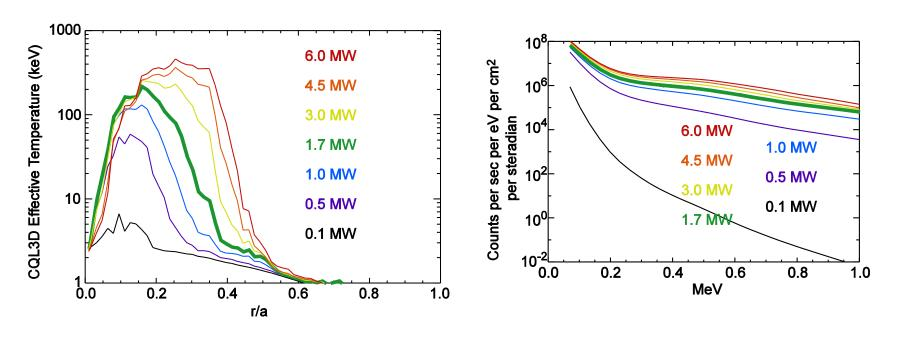
AORSA-CQL3D calculations of the fast ion temperature (left) and the estimated flux to the CNPA (right) as a function of RF power.
