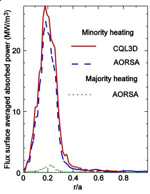
Convergence between AORSA and CQL3D can be determined by comparing the absorbed power calculated by each code.
