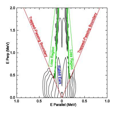
AORSA-CQL3D simulated midplane distribution at r/a = 0.3 shows a highly anisotropic fast ion distribution
