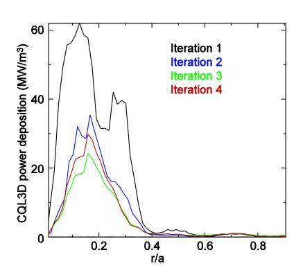
Convergence between successive runs of CQL3D occurs after 3-4 iterations. After which the absorbed power is seen to vary by ~10% between iterations.
